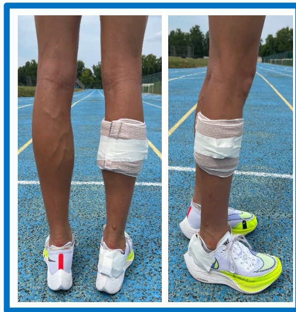
Figure 1. Frontal and sagittal view of the tibial and shoe-mounted IMUs during testing. Note: IMUs are shown secured with athletic tape to prevent extraneous movement.
